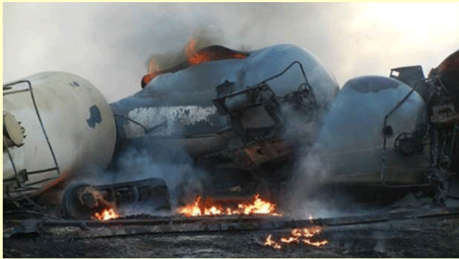
The above NTSB photo taken on December 31, 2013 shows part of the tank car pileup and residual fire resulting from the train collision the previous day near Casselton, North Dakota. The DOT-111 tank car in the center of the photo sustained a thermal tear and is still burning at the time.
